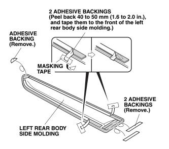
11. Align the left rear body side molding with the template, and attach it to the left rear door as shown.
