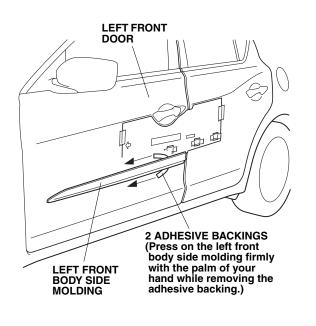
9. Using a rubber roller, apply firm pressure, especially at the ends, to set the adhesive.
